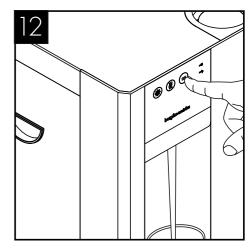
Pre-flush the new filter to waste using the ambient button until the water appears clear and is free of air. Flush through a small amount of water to check all functions.
