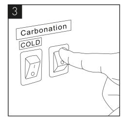
On sparkling models turn on the carbonation switch on the back of the unit.
