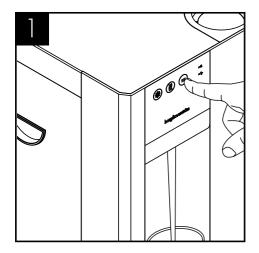
Briefly press chilled/ambient dispense buttons to release internal water pressure from the machine.
