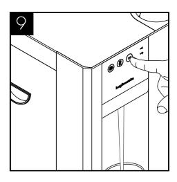
Leave the solution inside machine for sanitisation (minimum 5 minutes) while thoroughly cleaning the machine externally, pay particular attention to the dispense faucet and buttons.
