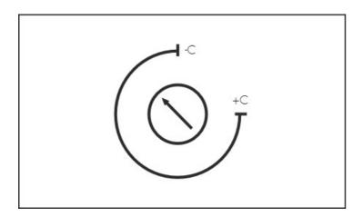
This shows the correct and factory default set point. Although adjustment is possible (clockwise reduces the temperature and anti-clockwise increases the water temperature), this correct default setting is to ensure optimum performance and reliability. Unauthorised alternative settings could cause technical issues and invalidate the warranty.
