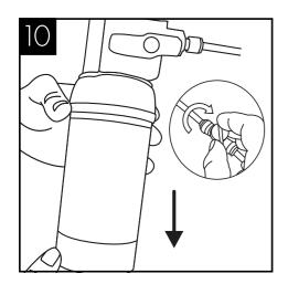
Turn off water and remove the service filter. Retain service filter for reuse.
