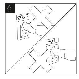
To avoid damage do not turn on the cold or hot power switches until water flows out of the machine. (If applicable)
