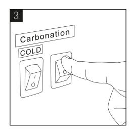
After completing the water installation, turn on the sparkling power switch and the pump will run. Do not open the regulator valve until the carbonated switch has been turned on.
