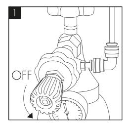
Attach the regulator to the disposable CO2 bottle, ensuring the regulator is closed.
