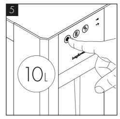
Flush through approximately 10 litres of sparkling water. Check and adjust the CO2 pressure accordingly.
