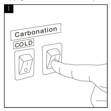
Switch off the Carbonation System switch on the back of the unit.
