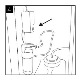
If enhanced Leak Detector is fitted as optional extra: locate the Leak Detector valve.
