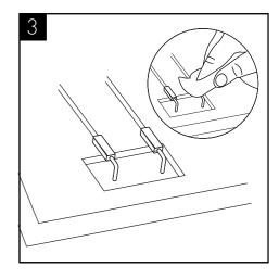
Locate the detection probe which can be found in the bottom rear middle section. Dry the probes and internal area with a dry cloth.
