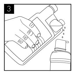
Add 25 ml of Sterizen® 30 Internal Water Cooler Sanitiser fluid to a clean and empty service filter cartridge.
